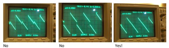
2. Repeat for IC2:14/PR22, IC3:7/PR32, IC3:14/PR42, IC4:7/PR52, IC4:14/PR62 until there are six perfect saw waves.
